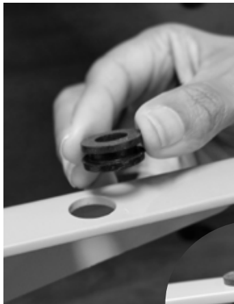
Step 3a: Insert Rubber Cushion
