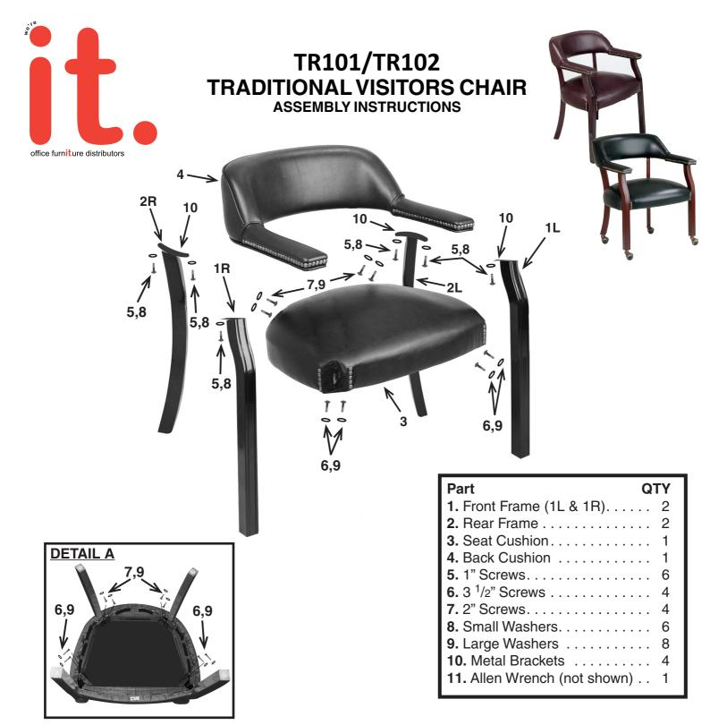
STEP 1 Remove all the parts from carton, separate them into part numbers indicated on the list and make sure part quantities are correct.
